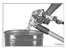
Remove nozzle from gun. Trigger gun into bucket until most of texture mix is pumped out. Allow water to flow through gun until gun is clean.
