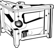
The adjustable corner finisher is used in conjunction with the corner applicator (model 35TT or 50TT) or the MudRunner ™(model 14TT) to apply the finish coat over the internal corners. The model 48TT can also be used to follow the corner roller and wipe down excess compound left when the tape is embedded in the corner. The spring action compensates for corners that are slightly over or under 90 degrees and the blade design produces smoothly feathered corners.
